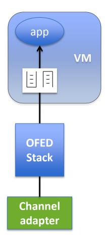
An RDMA Channel Adapter (IB HCA or iWARP rNIC) does the v-p-v translations automatically
