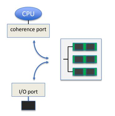
Choose the number of CPU cores to match the capacity of the I/O memory port (or vice versa)
