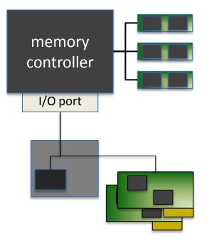
The I/O bus is designed to connect various I/O protocol adapters to host memory.
